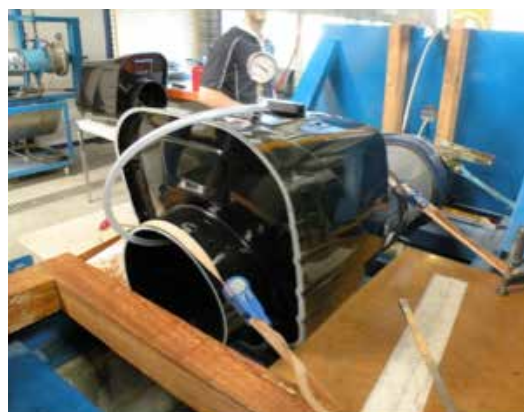
Validation of the resistance to pressure of a valve MULTI 315 . The same type of test is applied to all the MULTITUBE range.
